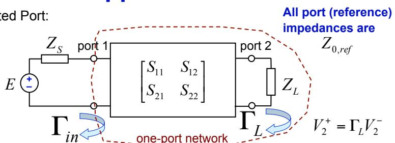
$$\Gamma_{in} = S_{11} + \frac{\Gamma_L S_{12} S_{21}}{1 - \Gamma_L S_{22}}$$
