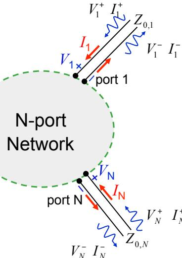
Note: all current components are defined positive with direction into the positive terminal at each port
