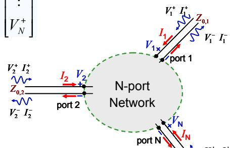
**Note:** S-parameters depend on port impedances  $Z_{0,n} = Z_0$
