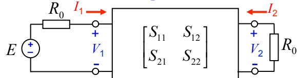
$$V_1^+ = \frac{1}{2}(V_1 + Z_0 I_1) \quad V_2^- = \frac{1}{2}(V_2 - Z_0 I_2)$$
