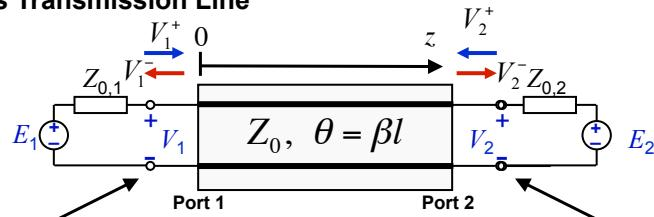
$$V_1 = V_1^+ + V_1^-$$
