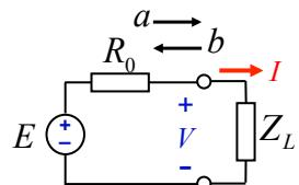
$$\begin{aligned} P_L &= P^+ - P^- = \frac{|V^+|^2}{2R_0} - \frac{|V^-|^2}{2R_0} \\ &= \frac{1}{2} \left\{ |a|^2 - |b|^2 \right\} \end{aligned}$$
