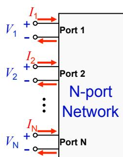
$$\begin{bmatrix} V_1 \\ V_2 \\ \vdots \\ V_N \end{bmatrix} = \begin{bmatrix} Z_{11} & Z_{12} & \cdots & Z_{1N} \\ Z_{21} & Z_{22} & \cdots & Z_{2N} \\ \vdots & \vdots & & \vdots \\ Z_{N1} & Z_{N2} & \cdots & Z_{NN} \end{bmatrix} \begin{bmatrix} I_1 \\ I_2 \\ \vdots \\ I_N \end{bmatrix}$$
