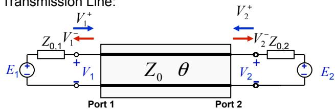
If  $Z_{0,1} = Z_{0,2} = Z_0$ , the scattering parameters can be easily obtained by inspection:
