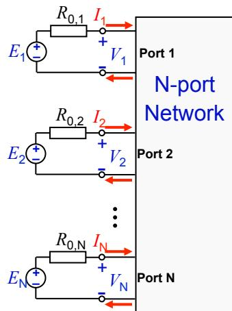
$$\begin{bmatrix} b_1 \\ b_2 \\ \vdots \\ b_N \end{bmatrix} = \begin{bmatrix} S_{11} & S_{12} & \cdots & S_{1N} \\ S_{21} & S_{22} & \cdots & S_{2N} \\ \vdots & \vdots & & \vdots \\ S_{N1} & S_{N2} & \cdots & S_{NN} \end{bmatrix} \begin{bmatrix} a_1 \\ a_2 \\ \vdots \\ a_N \end{bmatrix}$$
