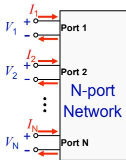
$$\begin{bmatrix} I_1 \\ I_2 \\ \vdots \\ I_N \end{bmatrix} = \begin{bmatrix} Y_{11} & Y_{12} & \cdots & Y_{1N} \\ Y_{21} & Y_{22} & \cdots & Y_{2N} \\ \vdots & \vdots & \ddots & \vdots \\ Y_{N1} & Y_{N2} & \cdots & Y_{NN} \end{bmatrix} \begin{bmatrix} V_1 \\ V_2 \\ \vdots \\ V_N \end{bmatrix}$$
