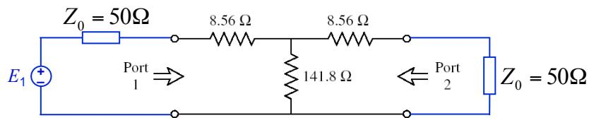
$$V_1 = E_1 \frac{Z_{in,1}}{Z_{in,1} + Z_0} = \frac{1}{2} E_1 \quad Z_{in,1} = 41.444 \Omega + 8.56 \Omega \approx 50 \Omega$$
