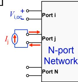
**Open-Circuit Impedance Parameters**
