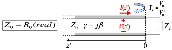
$$V(z') = V_0^+ (e^{+j\beta z'} + \Gamma_L e^{-j\beta z'})$$
